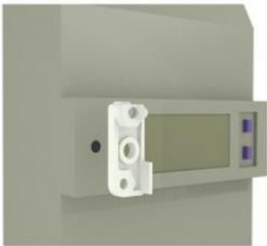
If it is an **electronic meter**, stick the adhesive plastic mount on the meter in front of the meter blinking light (aim through the hole)
